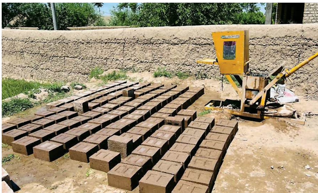
Image 9: Production of compressed stabilized mud blocks through manual machines within the community by the owners of shelters
