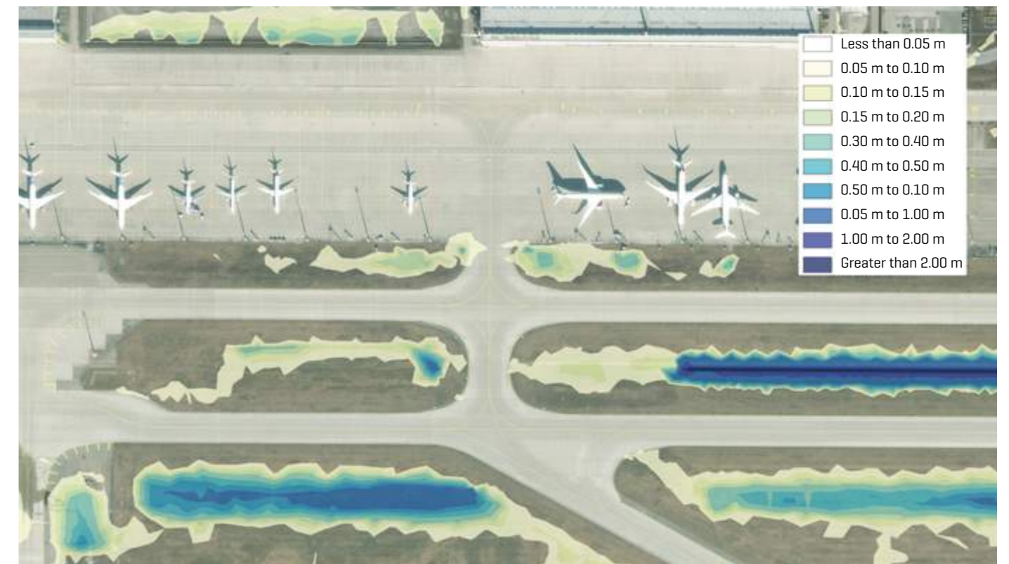
Extract from the hydrodynamic drainage simulation model showing the calculated flooding in the event of heavy rainfall [60 mm/h].
